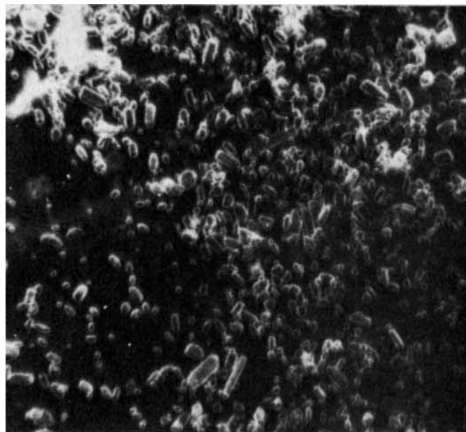
Figure 9—Micrograph of tolbutamide particles released from a coprecipitated dispersion of tolbutamide (10% w/w) and II into aqueous sodium chloride solution (0.9% w/w) previously saturated with tolbutamide (×100).
